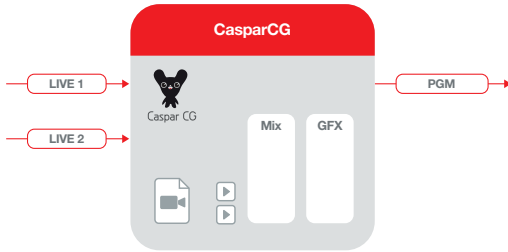
Example 4: Integrated Channel Playback Full channel capability including live inputs, clip players, and graphics overlay
